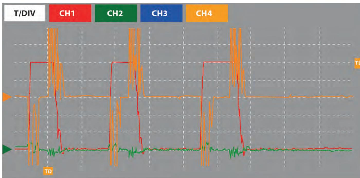
CH4 Freq: 73.5 kHz D.Cycle: 49% Nivel Trigger: 1.92 A
